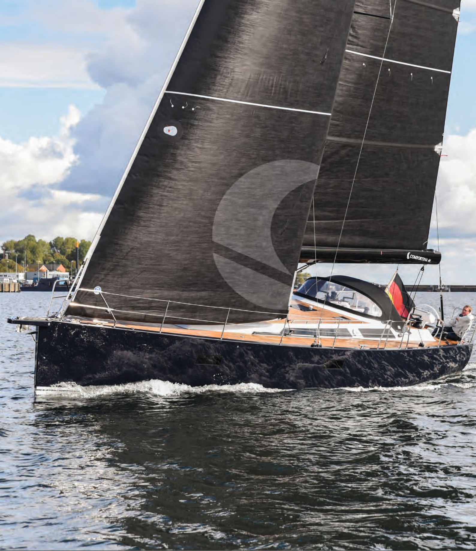
COMFORTINA 46 WERFT: COMFORTINA GMBH & CO KG DESIGN: DIETER BLANK YACHTDESIGN MATERIAL: GURIT AMPREG™ 30, CORECELL 80-130KG, SPABOND™ 340, SPABOND™ 568. SELCOM E-GLAS, GURIT CARBON UD'S
